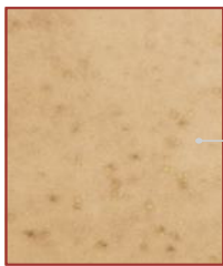
CuSn8 with Composition Sn 8 % P < 0,05 % Cu Rest
